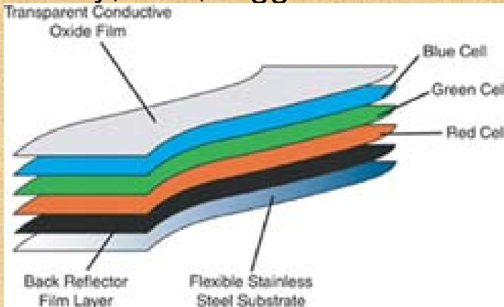
UniSolar a-Si cell structure. Source: <http://www.unisolar.com/interior.asp?id=67>
