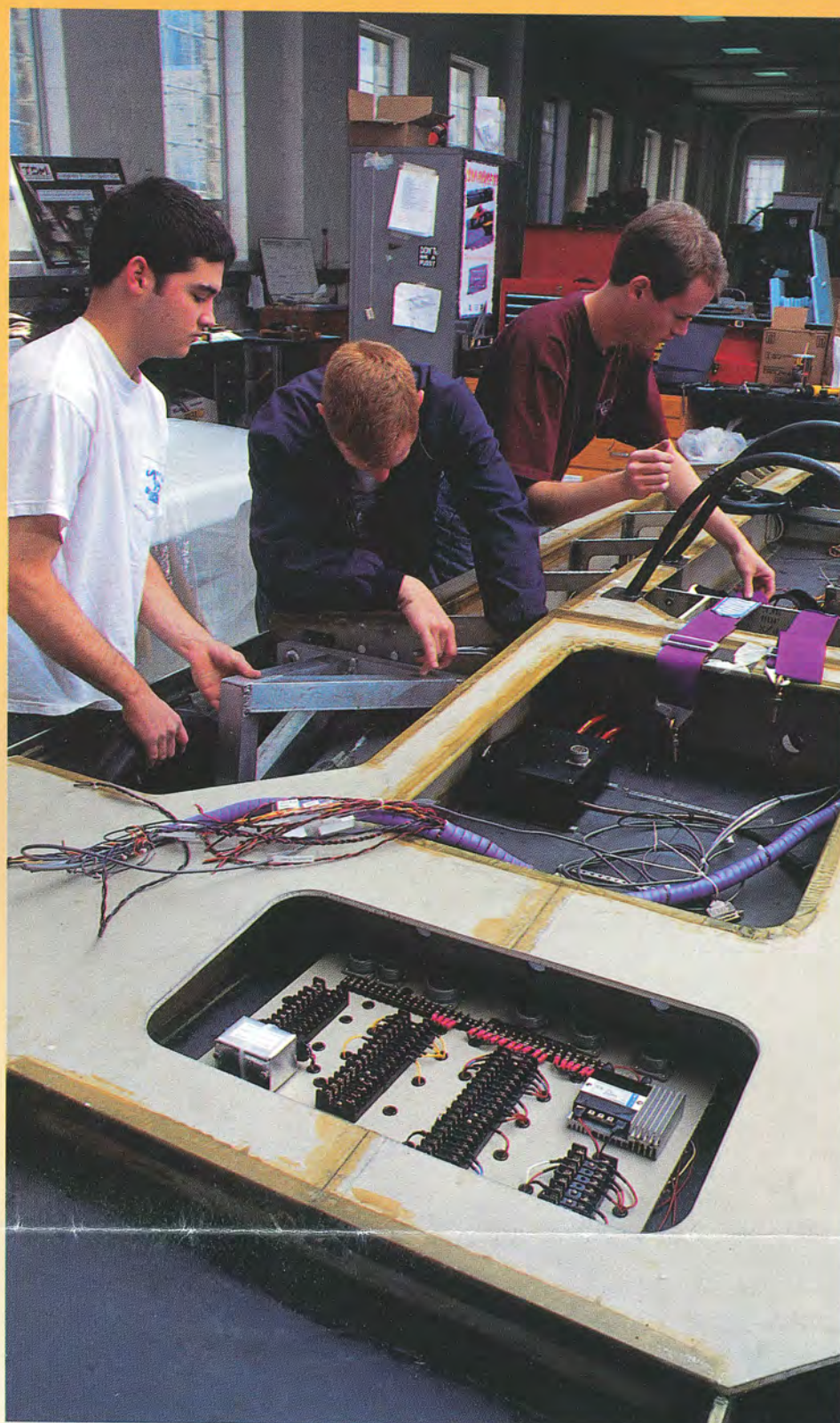
Jason Northup, left, and Damian Brandenburg, center, drop a rear wheel assembly into place while Chris Hopkins makes an adjustment to wiring for cockpit controls.
